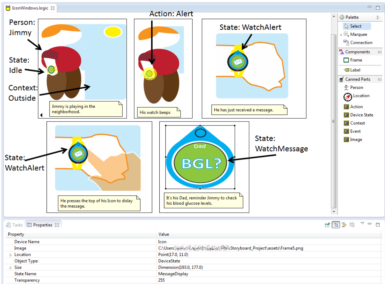
Figure 3: Screenshot of electronic storyboarding tool in Eclipse showing an example storyboard, palette, and properties view. Arrows indicate the type of tagged object and its value.
