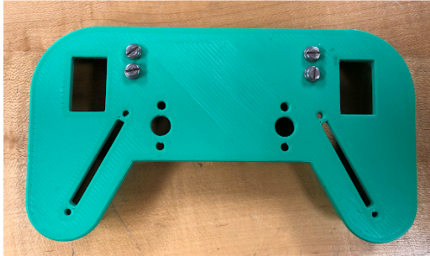
Figure 2: Ebot handheld controller shell
