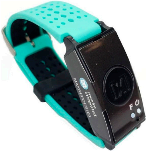
Figure 3. Maxim Integrated Wearable Device. Note. The Maxim Integrated MAXREFDES103 was used to detect user HR and HRV throughout the experiment.
