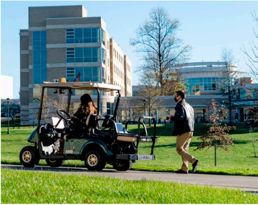
Figure 4. Testbed environment in action. Note. The figure shows the JMU autonomous vehicle traveling on a walking path with a “safety officer” following to manually turn off the vehicle if needed.
