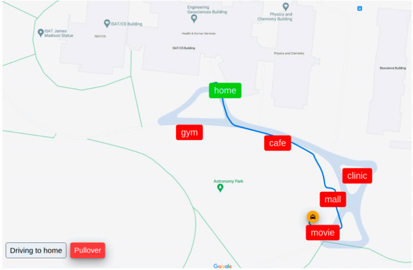
Figure 2. Graphical User Interface. Note. GUI for autonomous vehicle showing selectable destinations, vehicle position, destination, and pull-over controls.
